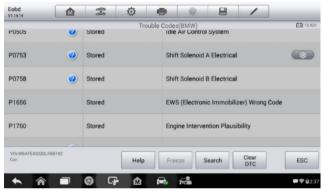
Figure 4-16 Sample DTC & FFD Screen
