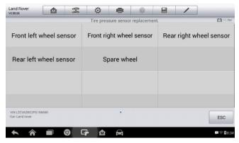
Figure 5-31 Sample Tire Pressure Sensor Replacement Screen
